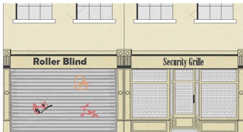
Figure 5: The roller blind on the left, obscures visibility into the shop, which compromises security and is a target for graffiti. The security grille on the right is more sympathetic to the traditional character of the shopfront, and enables visibility into the premises
